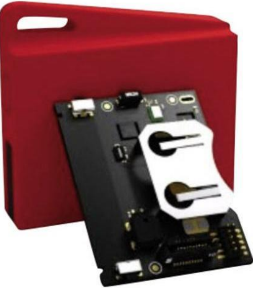
Prototypingkit Texas Instruments CC2650STK
